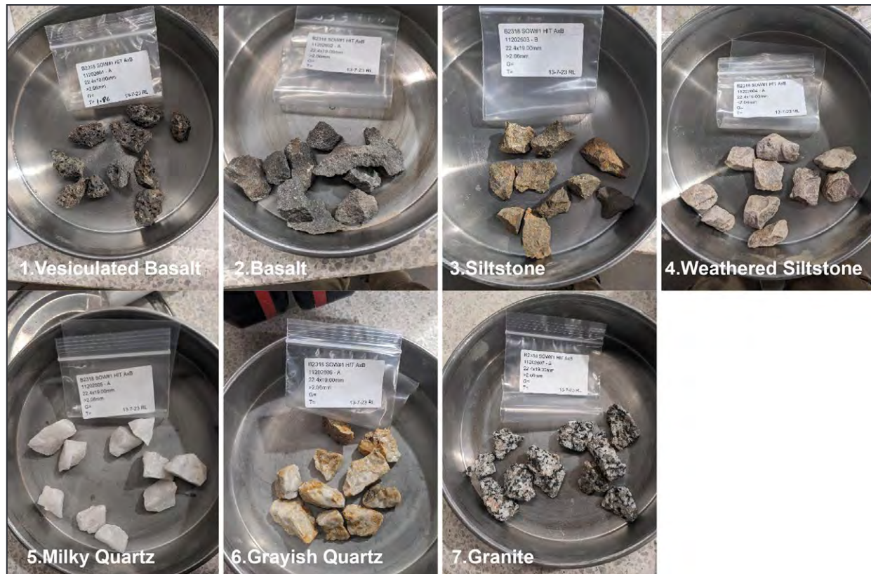
Figure 4. Images of 10 fragments in the 22.4×19 mm size fraction used in HIT Axb tests
