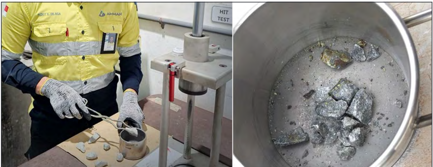
Figure 1. Image of HIT device and close-up of broken rock in cup
